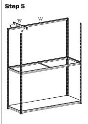
Fix brackets 'B' at the very top allowing room for the MDF board to sit flush against the legs. Repeat with brackets 'A'.
