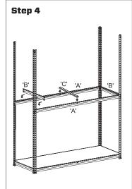
Fix brackets 'B' so that the top rivet sits on the upper legs and the bottom rivets sit on the lower legs. Repeat with brackets 'A', followed by brace 'C' as shown
