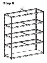
Apply remaining brackets as above to desired height. Ensure that braces 'C' are fixed to all shelves
