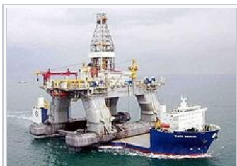
The Deepwater Nautilus , sister rig to the Deepwater Horizon being transported aboard a heavy-lift ship
